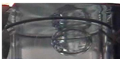
Fig. 7. Experimental results for 1-g (heat input: 3.2 W, 2.13 \times 10^8 \text{ W/m}^3 ) and low-g (heat input: 15 W, 1000 \text{ W/cm}^3 ) environments.
